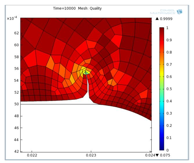
At the edges I get crazy pointy shapes like this. (the curved section is masked, so it does not receive any deposit)
