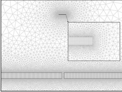
**Figure 2** Mesh profile of the structure. Inset shows close-up of the nanotube tip.
