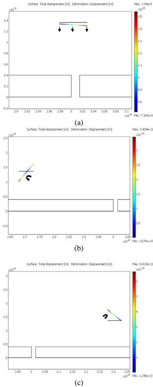
**Figure 7** Effect of initial orientation on movement (a) Nanotube directly above the microelectrodes tips moving down directly; (b) Nanotube rotating on the left of the tips; (c) Nanotube rotating on the right of the tips.
