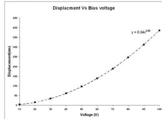
**Figure 5** Simulated nanotube displacement vs bias voltage (big dots). The equation for the curve fit (dash line) is also shown.
