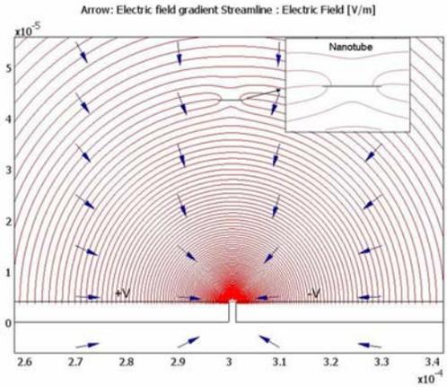
**Figure 3** The electric field distribution. Streamlines show electric field and solid arrows indicate the electric field gradient (NOTE: Arrow lengths do not represent magnitude of the electric field gradient). Inset shows the electric field distorting around the nanotube.
