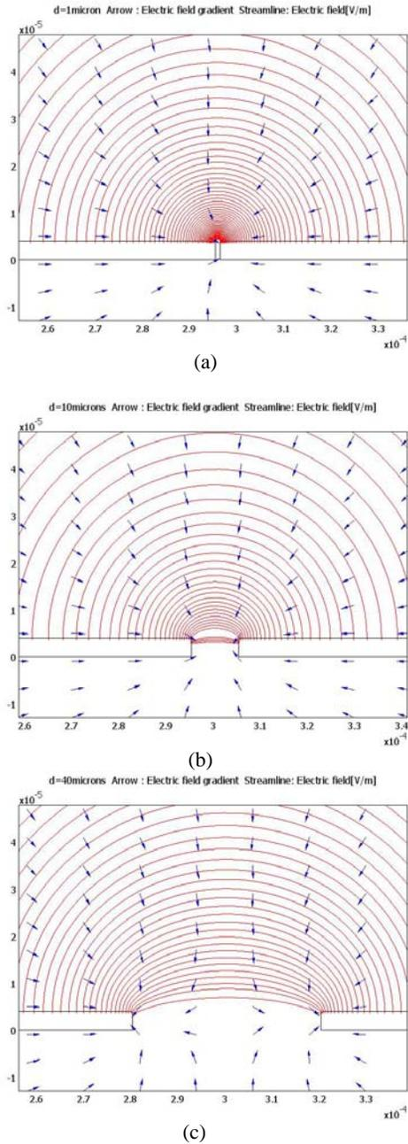
**Figure 4** Streamline plot of electric field lines close to the electrode tips. The arrows indicate the direction of electric field gradient (a)  $d=1\mu\text{m}$ ,  $E_{\text{max}}=2.3\text{E}+8\text{ V/m}$ ; (b)  $d=10\mu\text{m}$ ,  $E_{\text{max}}=5.0\text{E}+7\text{ V/m}$ ; (c)  $d=40\mu\text{m}$ ,  $E_{\text{max}}=4.8\text{E}+7\text{ V/m}$
