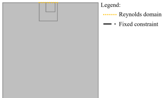
Figure 2: EHL computation domains at the contact scale.
