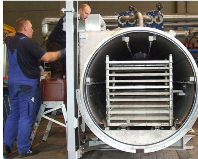
Thermal sterilization using Retort
