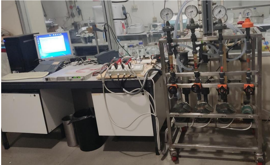
ED plant control station
