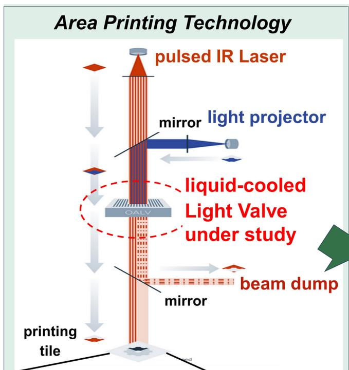
**Figure 1.** Area Printing on a metal powder bed. A liquid-cooled light valve is used for dynamic beam patterning. Near 100kW Infrared (IR) patterned beam melts powder layer by layer.
