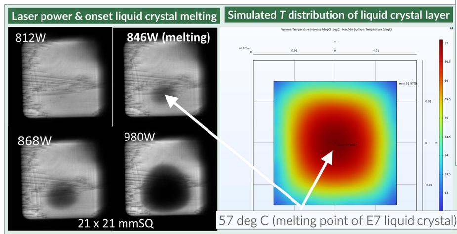
**Figure 2.** Experimental validation of COMSOL FE model of light valve laser heating. The threshold laser power for E7 liquid crystal phase transition<sup>2</sup> at 57°C appears as a dark spot in cross-polarizer image, consistent with calculations presented.
