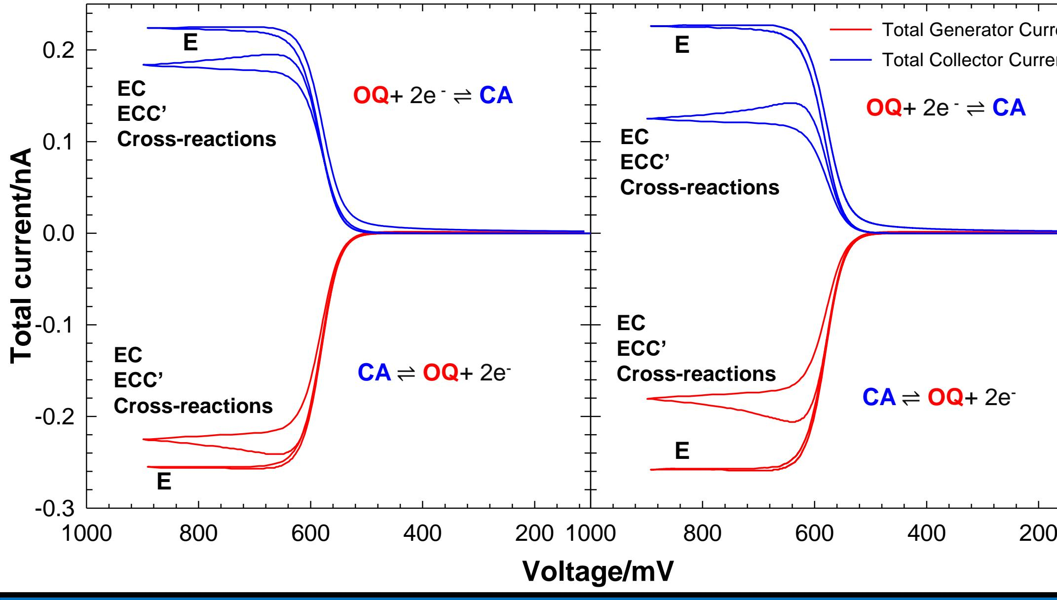
EC, ECC', and cross reactions in a mixture of DA and NE show no significant difference in their currents due to the close proximity of the electrodes. DA and NE do not have enough time to undergo an ECC' mechanism to play a role in the overall of the reaction.
