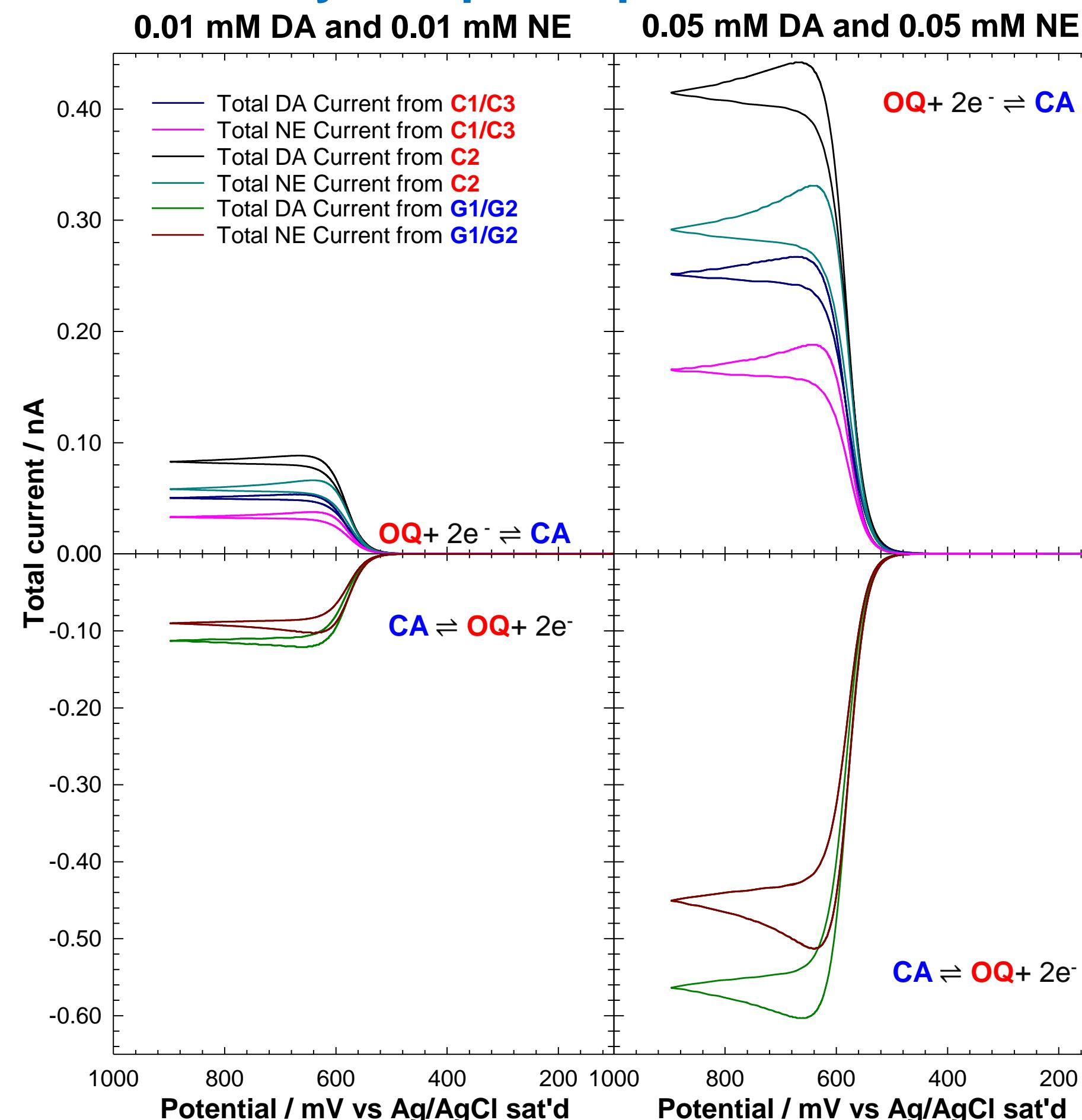
DA and NE cannot be differentiated at a gap of 4  $\mu\text{m}$ .
