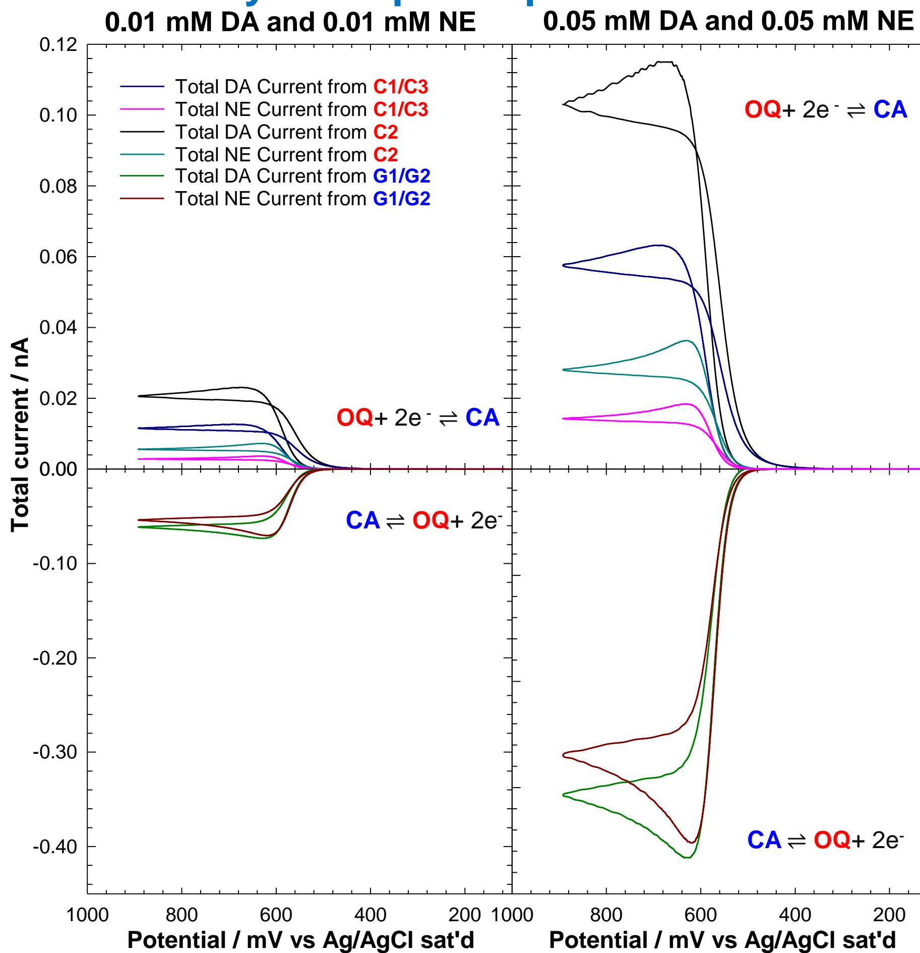
The differentiation of the catecholamines becomes possible at a gap of 20  $\mu\text{m}$  and 0.01 of DA and NE.
