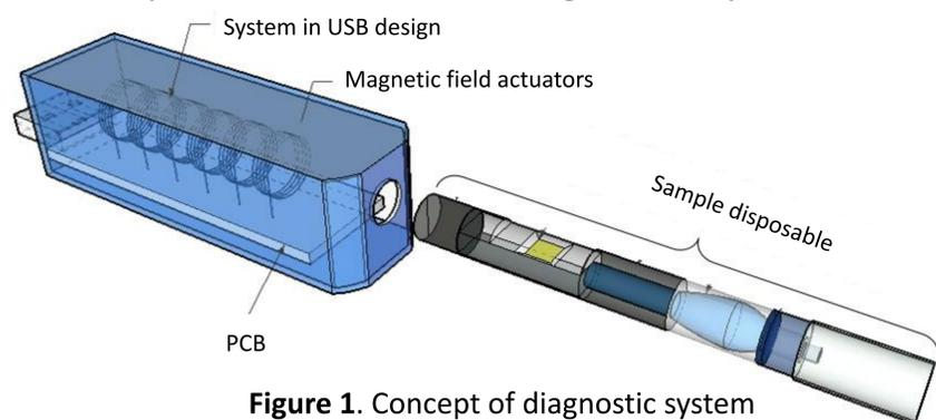
Figure 1. Concept of diagnostic system
