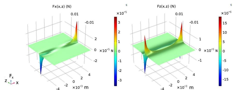
Figure 3. Magnetic forces in radial ( $x$ ) and height ( $z$ ) direction
