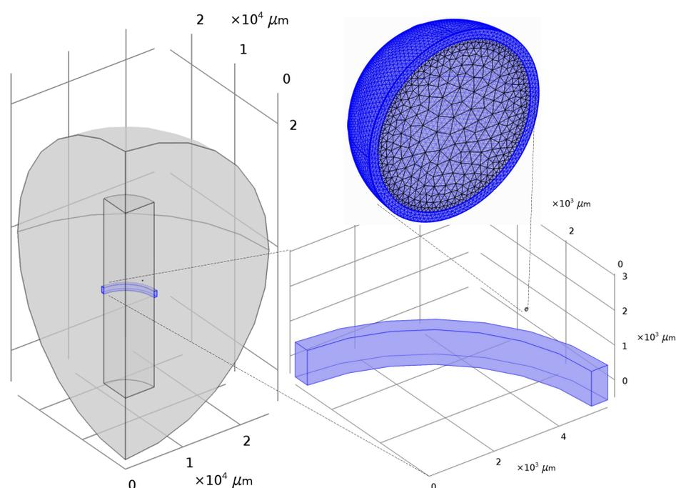
Figure 2. Quarter model, zoomed inductor and bead with magnetic coating
