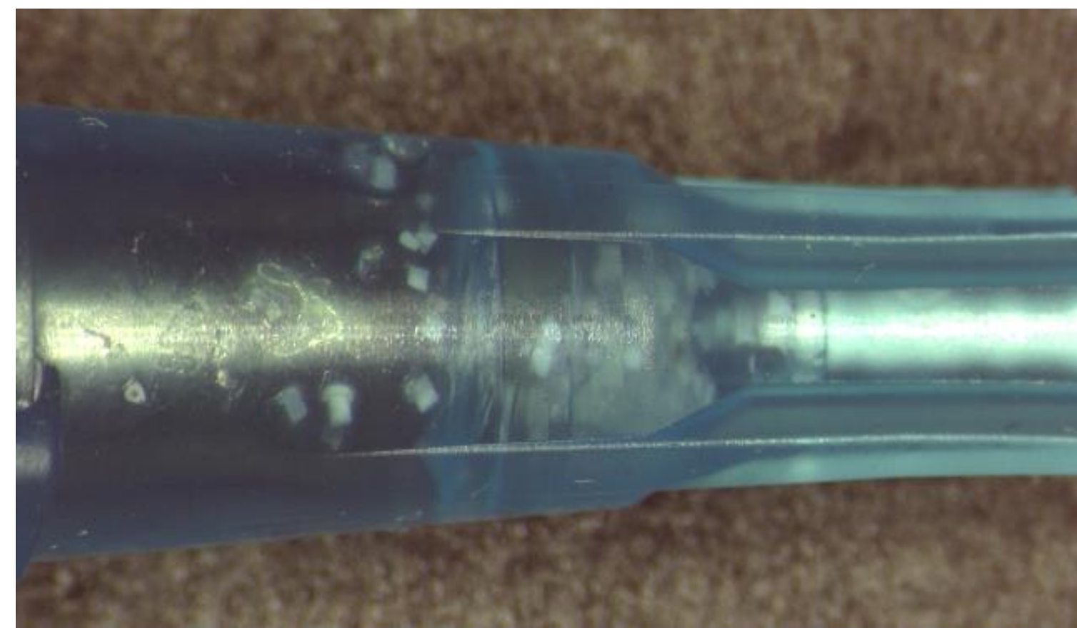
Figure 1. An example of unsuccessful transfer of microparticles (white) during injection with a hypodermic needle
