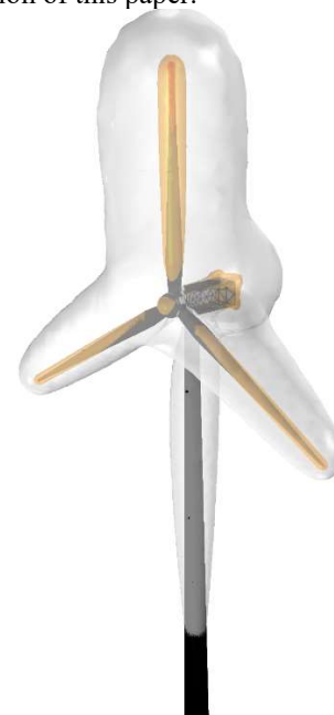
Figure 1 – Illustration of electric field around wind turbine. The highest field is located at the tip of the upward facing blade (red), The mid-span part of the blade and the end of the nacelle are characterized by medium field areas (yellow). The tower and the inner side of the nacelle are characterized by low electric field magnitudes (white).
