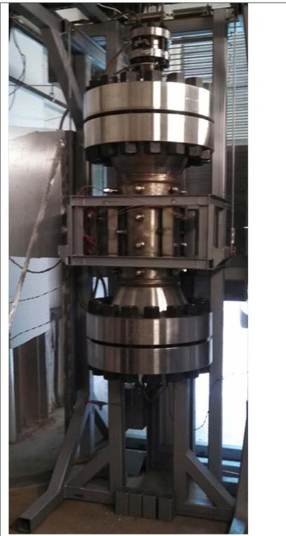
Figure 1. Overpressure furnace
